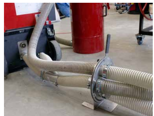
Mobile insertion using switchover function between blowing and suction operation
