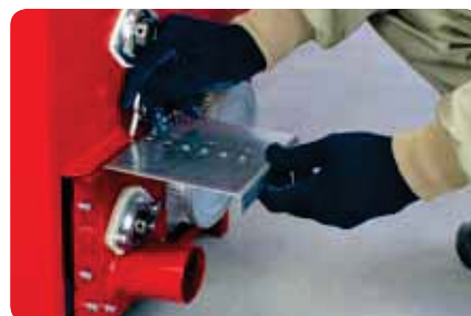
Setting of the airlock feed gate
